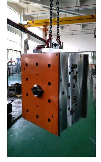
Is the mold clean and free of debris and rust 模具是否清洁干净没生锈
